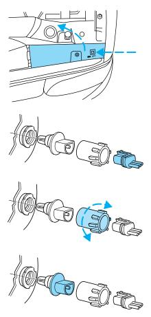
2. Disconnect the electrical connector from the bulb by pulling rearward.
